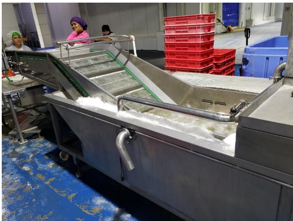
Figure 83: Mechanical Drying End of the Glazing Unit
