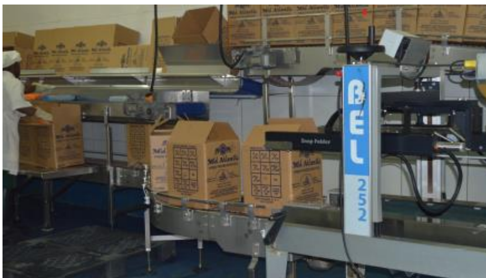
Figure 48: Unsealed Cartoon Boxes Passed Through Snap Fold Machine
