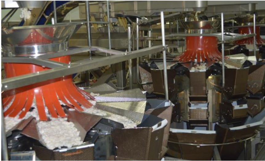
Figure 35: Dispersion Feeders of Installed Automated Packaging System
