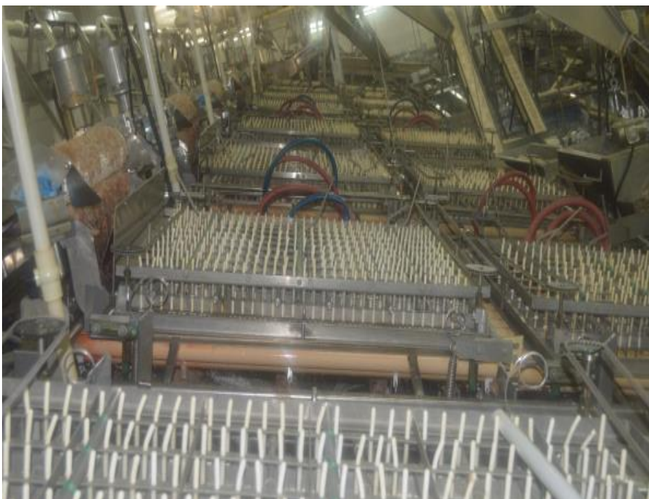
Figure 24: Automatic Mechanical Shrimp Peeler System
