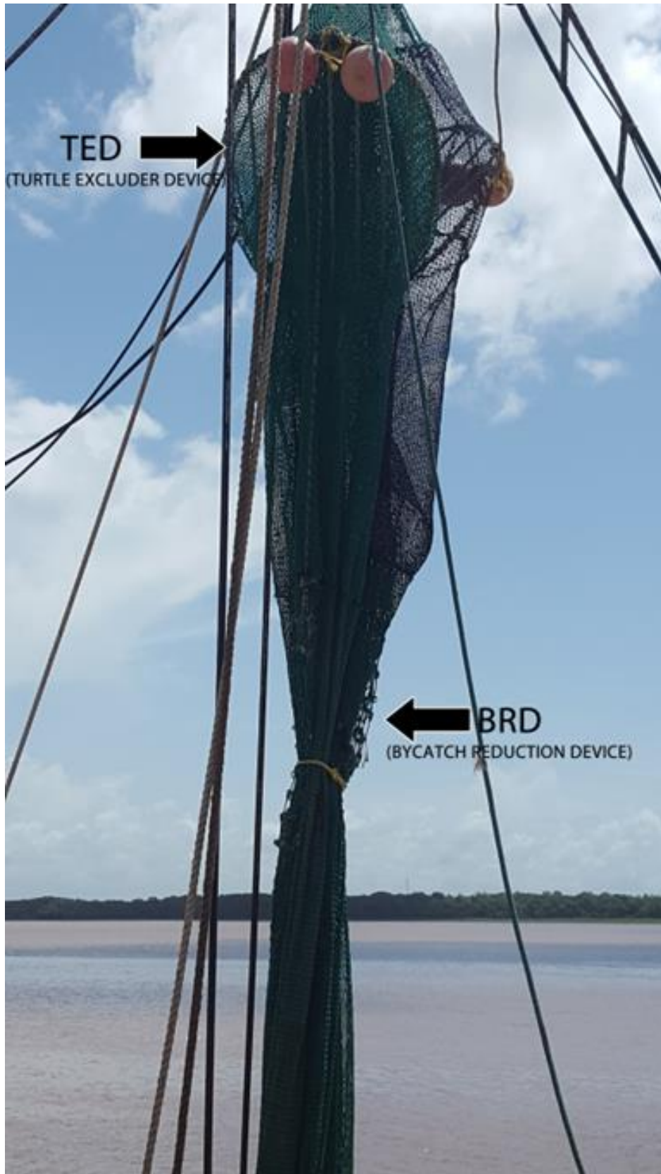
Figure 13: Turtle Exclusion and Bycatch Reduction Devices on Trawling Gear
