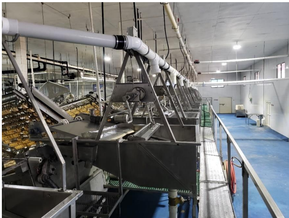
Figure 22: Automatic Mechanical Peeler System
