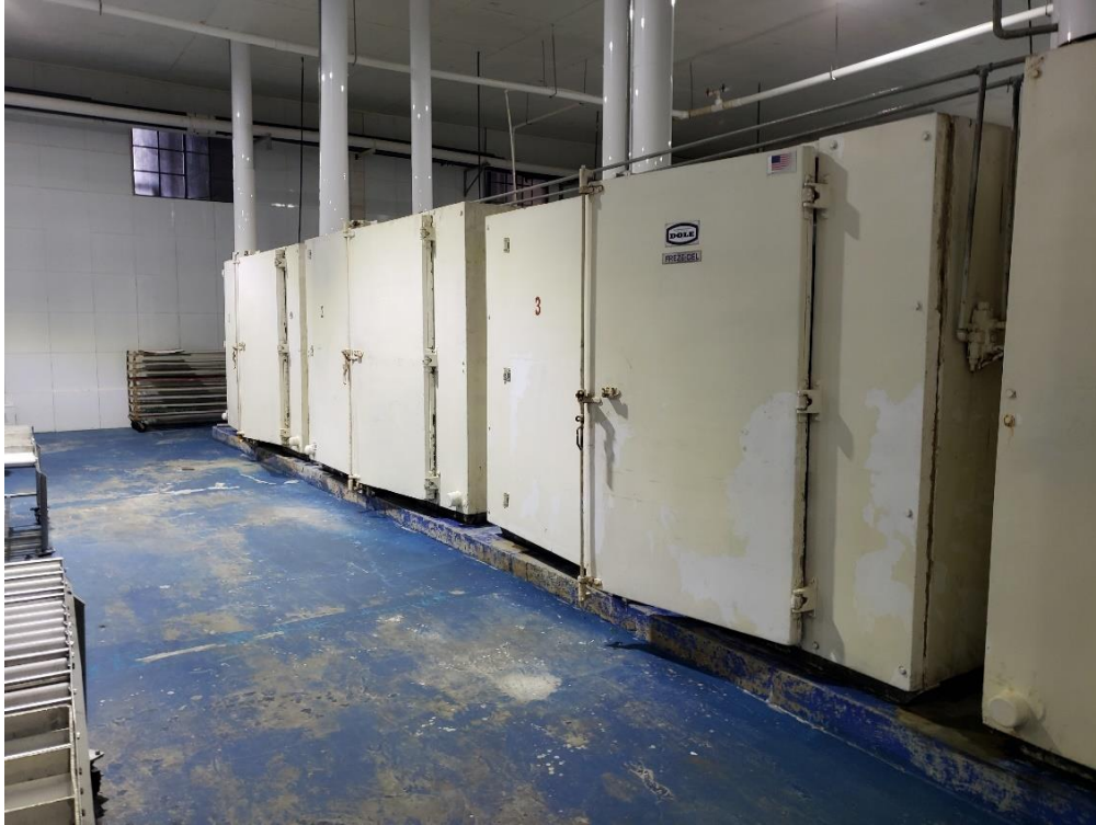
Figure 40: Plate Freezers in Freezing Area
