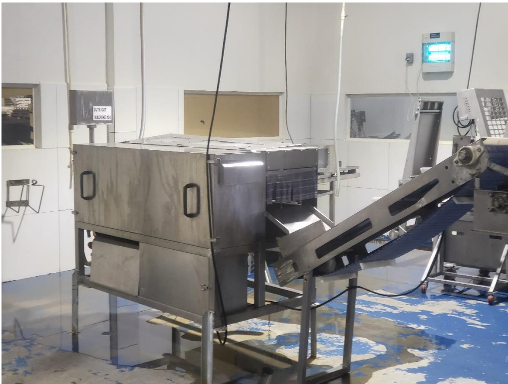
Figure 71: Degutting Machine
