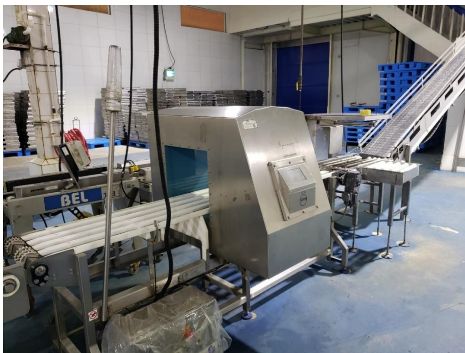
Figure 49: Metal Detection System
